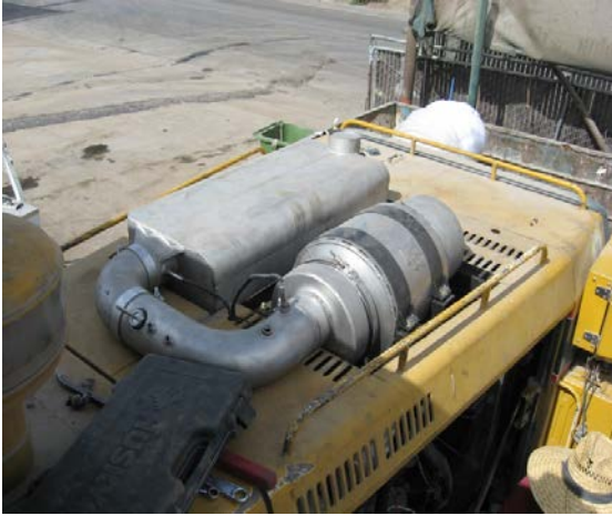
DPF and SCR Catalyst on Loader
