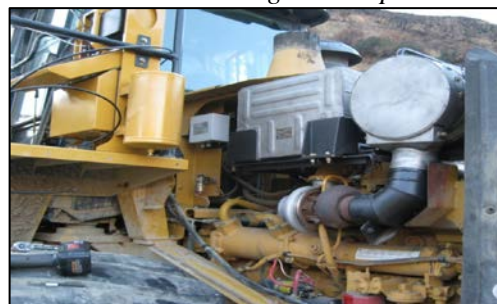
DPF and SCR in Engine Compartment
