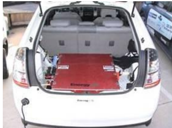
Figure 13: EnergyCS battery integrated in a passenger vehicle
