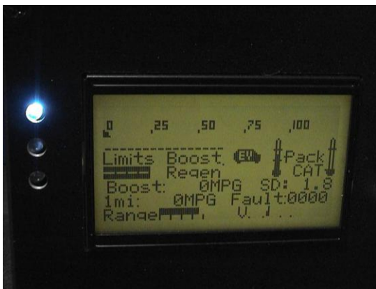
Figure 12: EnergyCS display includes battery voltage and temperature
