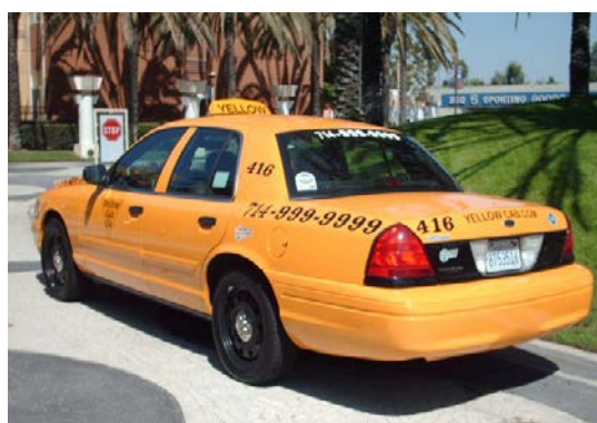
Converted CNG-Fueled Taxicab
