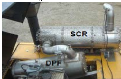
ServoTech DECS Mounted in Place Above Engine on Excavator Vehicle
