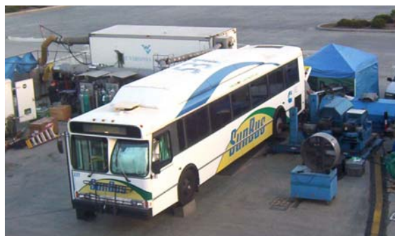
Figure 1 Transit Bus on WVU Transportable Heavy-duty Chassis Dynamometer
