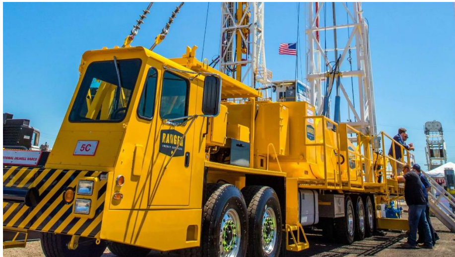
Figure 3: A Workover Rig in the Field
