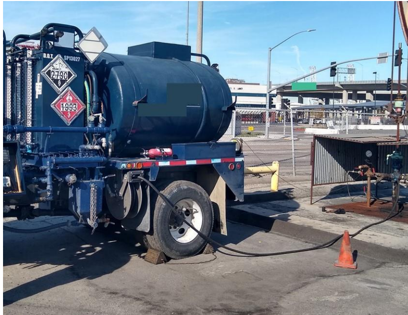
Figure 2: Chemical Delivery from a Treater Truck to a Well
