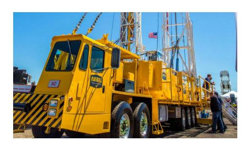
Shown in the picture is an example of a workover rig. It is commonly used to perform maintenance on an oil well and can be used to remove and/or replace tubing.
