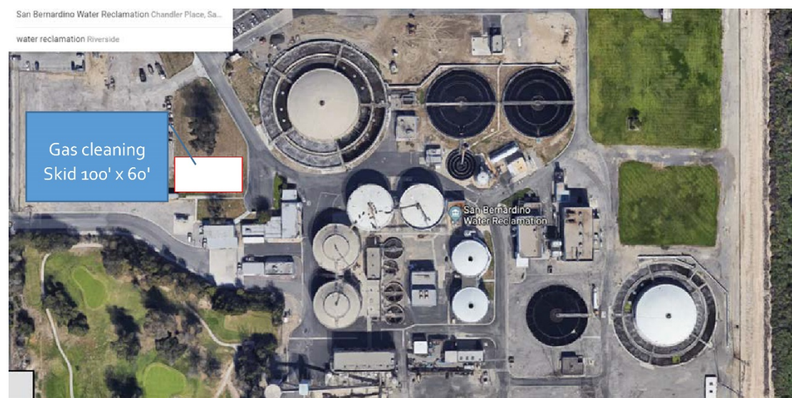
Figure 15 Proposed Site Plan for Gas Conditioning Skid
