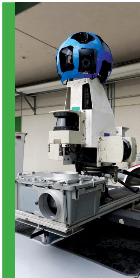
Google camera with enclosure box for low-cost sensors
