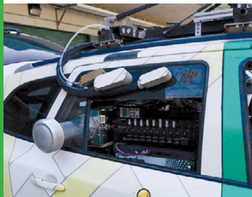
View of sampling duct, power control panel, and data logger
