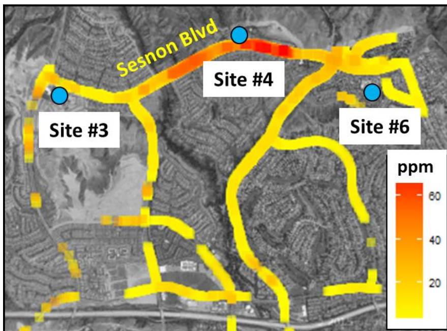
Figure 2. Map of the highest methane concentrations measured by the SCAQMD's mobile monitor between 12/21/2015 and 1/29/2016.
