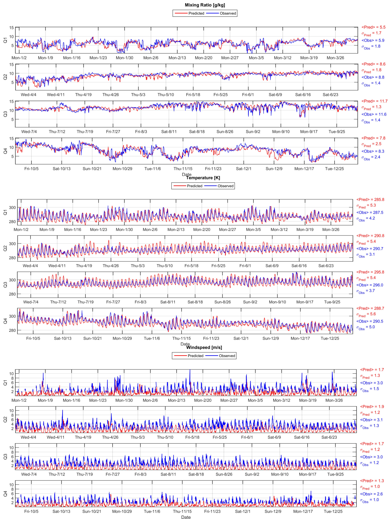
Figure 12: Time Series of Measured and WRF Simulated Mixing Ratio (Top), Temperature (Middle), and Wind Speed (Bottom) for the Period of Jan 1 to Dec 31, 2012 at John Wayne-Orange County Airport
