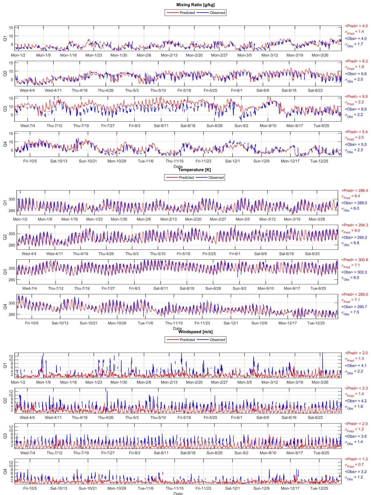
Figure 10: Time Series of Measured and WRF Simulated Mixing Ratio (Top), Temperature (Middle), and Wind Speed (Bottom) for the Period of Jan 1 to Dec 31, 2012 at San Bernardino International Airport
