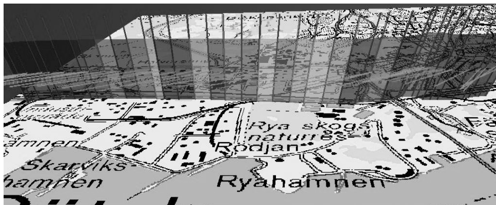
Figure 1. A 3D plot of a SOF measurement conducted at the oil harbor. The lines correspond to the solar light, which together with the movement defines the area cut out through the atmosphere.
