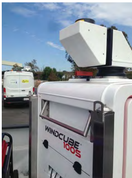
Figure 8. The WindCube 100S (Leosphere) LIDAR used for wind profile measurements in this project.
