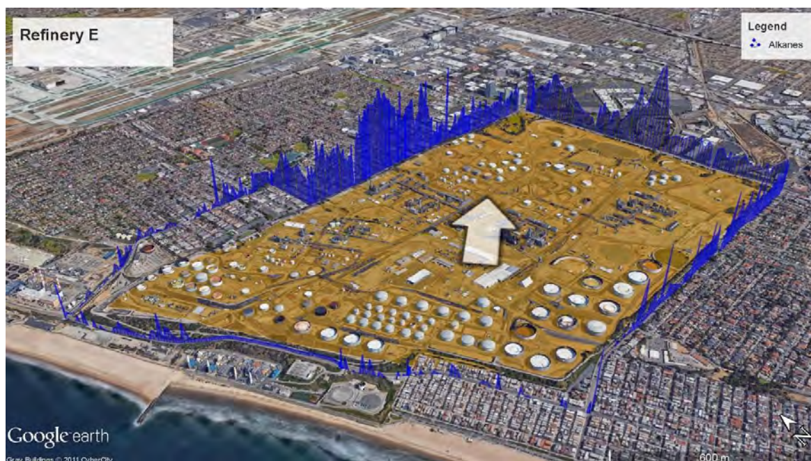
Figure 42. Example of a SOF ‘box’ measurement of Refinery E (orange area) 6 November 2015, 10:47-11:22. Alkane column is shown as a blue curve with apparent height proportional to gas column (10 m equivalent to 1 mg/m 3 , max 55 mg/m 3 ). Wind direction during the measurement is indicated by the white arrow. Average wind speed during this particular measurement was 1.8 m/s. Emissions on the upwind side are subtracted from the downwind side in order to get emissions from within the box. This particular transect measured 229 kg/h from Refinery E.
