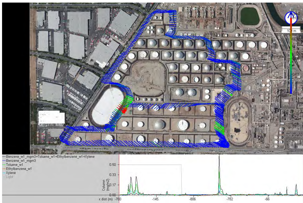
Figure 60. Aromatic VOC concentrations in mg/m 3 across the tank farm measured using MWDOAS. Bars are pointing towards the wind, hence in the direction of the source. North is upwards in the figure.
