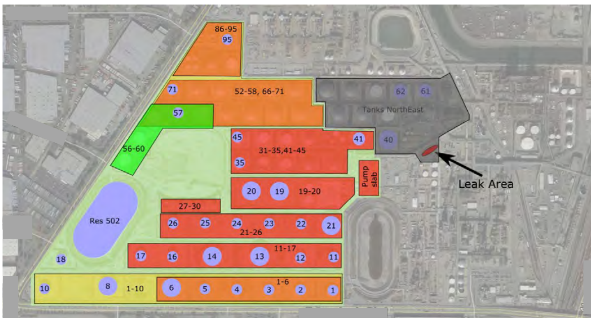
Figure 52. Overview of the tank farm part of the refinery where on site measurements with SOF + MeFTIR + MWDOAS were conducted for about one week in September/October 2015. Tanks, tank groups and specific areas have been given numbers and names respectively for reference to measurement results. North is upwards. Groups of quantified tanks are denoted by coloured rectangles, and individual tanks that have been quantified are indicated by blue shapes/circles. The surveyed part (large light green area) is restricted in the west and south by the site fence-line, and in the east and north by roads going east of tank 1-11-21-Pump slab and then between the “Tanks NorthEast” and tank groups “52-58+66-71” and to the northeast corner of group “86-95”.
