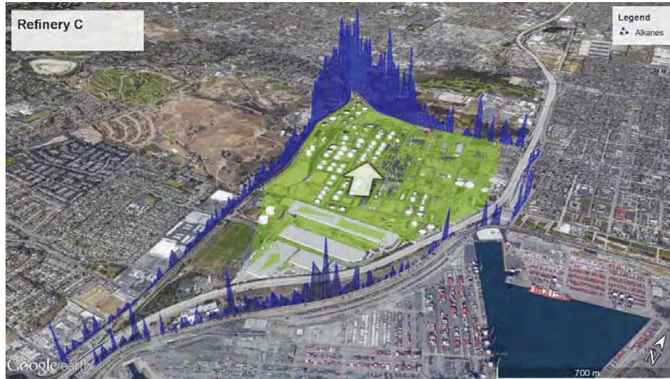
Figure 30. Example of a SOF 'box' measurement of the Refinery C (green area) 7 September 2015, 11:57-12:18. Alkane column is shown as a blue curve with apparent height proportional to gas column (10 m equivalent to 1 mg/m 2 , max 76 mg/m 2 ). Wind direction during the measurement is indicated by the white arrow. Average wind speed was 2.9 m/s for this particular measurement. Emissions on the upwind side (from LA harbor) are subtracted from the downwind side in order to get emissions from within the box. This particular transect measured 285 kg/h from Refinery C.
