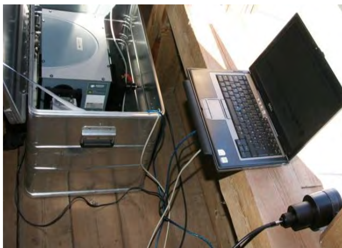
Figure 5. The mobile Sky-DOAS system: Telescope, optical fibre, spectrometer and control computer.
