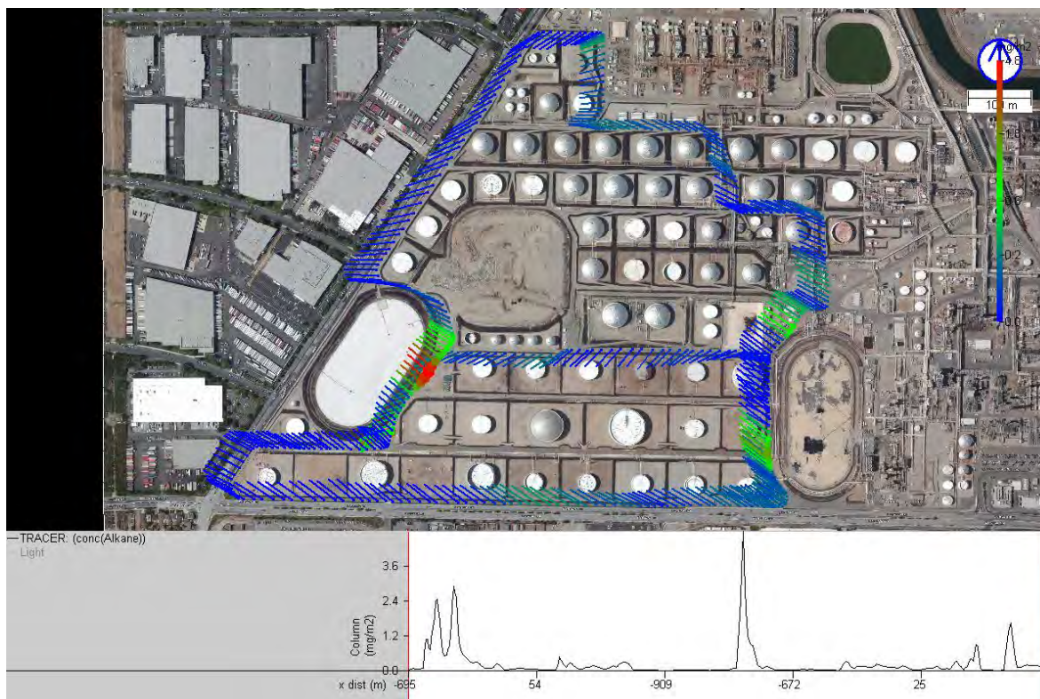
Figure 61. Alkane concentrations in \text{mg}/\text{m}^3 measured using MeFTIR across the tank farm. Bars are pointing towards the wind, hence in the direction of the source. North is upwards in the figure.
