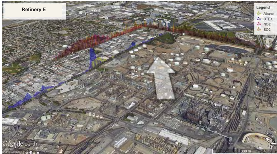
Figure 45. Transects of plumes originating from Refinery E: NO 2 (pink), SO 2 (brown), BTEX (blue) and alkane (yellow). NO 2 and SO 2 show column thickness and are both on the same scale (max NO 2 = 5.9 mg/m 2 , flux NO 2 = 42.5 kg/h, max SO 2 = 6.4 mg/m 2 , flux SO 2 = 48.9 kg/h), alkanes and BTEX show concentrations and are scaled independently for visibility (max BTEX = 0.04 mg/m 3 , max alkanes = 0.13 mg/m 3 ). Example transects from September 16, 4:23 PM and 9:07 PM.
