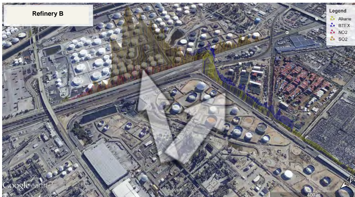
Figure 27. Transects of plumes originating from Refinery B. NO 2 (pink line) and SO 2 (brown line) were impacted by westerly winds (4.3 m/s). Conversely, BTEX (blue line) and alkane (yellow line) plumes were measured in the presence of northerly winds. The column thickness for both NO 2 and SO 2 is reported on the same scale (max NO 2 = 5.6 mg/m 2 , flux NO 2 = 11.7 kg/h, max SO 2 = 25 mg/m 2 , flux SO 2 = 68.2 kg/h). Alkanes and BTEX columns are scaled separately for better visibility (max BTEX = 0.03 mg/m 3 , max alkanes = 0.36 mg/m 3 ). The examples shown here were collected on September 8 and on September 19, 2015.
