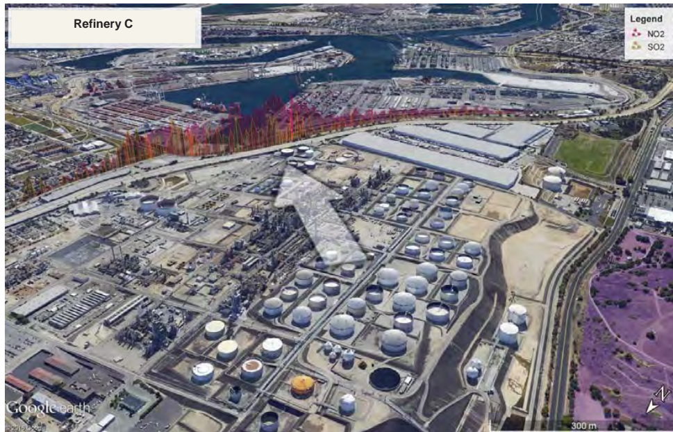
Figure 33. Transects of plumes originating from Refinery C. the NO 2 (pink) and SO 2 (brown) plume from Refinery C in north-westerly wind (3.7 m/s). Max NO 2 = 9.5 mg/m 2 , flux NO 2 = 81 kg/h, max SO 2 = 5.6 mg/m 2 , flux SO 2 = 37.5 kg/h Data from September 18 2:59 PM.
