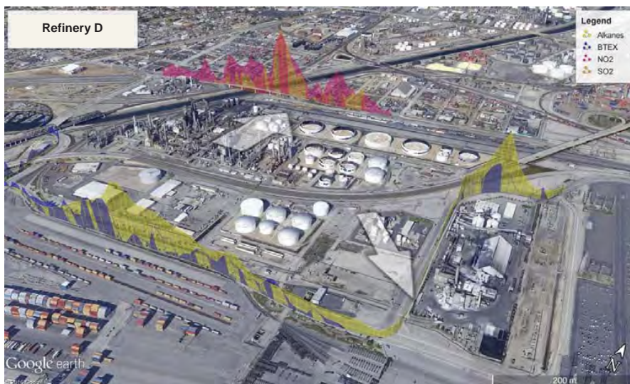
Figure 39. Transects of plumes originating from Refinery D: NO 2 (pink), SO 2 (brown) in south wind and BTEX (blue) and alkane (yellow) in north-westerly winds. NO 2 and SO 2 show column thickness and are both on the same scale (max SO 2 = 10.1 mg/m 2 , flux SO 2 = 18.3 kg/h, max NO 2 = 9.8 mg/m 2 , flux NO 2 = 39.3 kg/h), alkanes and BTEX show concentrations and are scaled independently for visibility (max BTEX = 0.02 mg/m 3 , max alkanes = 0.29 mg/m 3 ). Data from September 19, 12:42 PM and 8:32 PM.
