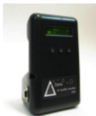
Customized low-cost optical particle counter
