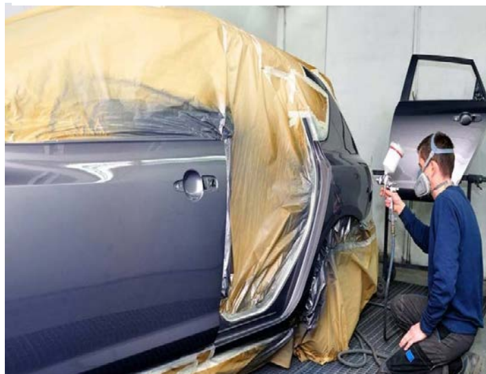
Figure 4-9: Application of Automotive Coating Inside a Paint Spray Booth
