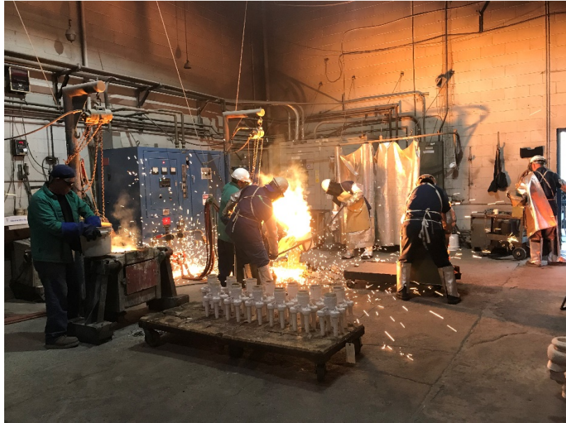
Figure 4-7: Pouring Molten Metal into Molds
