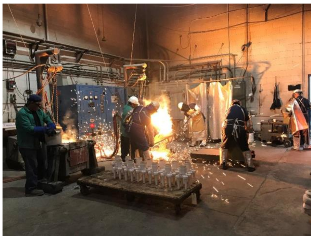
Figure 4-7: Pouring Molten Metal into Molds
