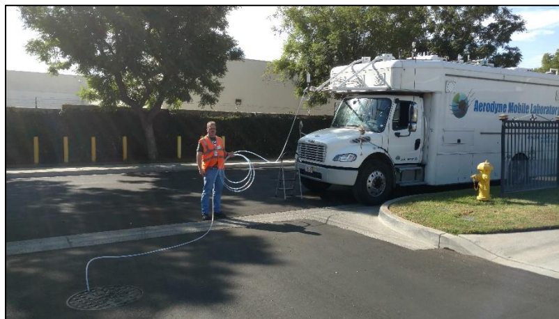
Figure 1. Sampling the headspace of a manhole using an extended inlet (‘snorkeling’).
