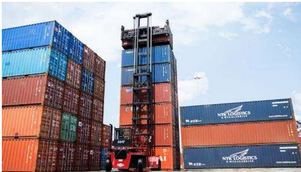
Figure 21: POLB Demonstrated Battery Electric Top Handlers and Yard Tractor, and a Fuel Cell Yard Tractor
