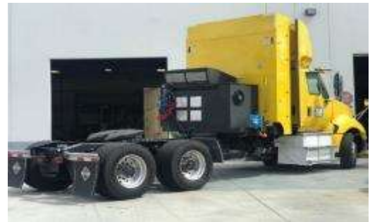
Figure 17 TransPower’s PHET-2 Rear Mounted ICE
