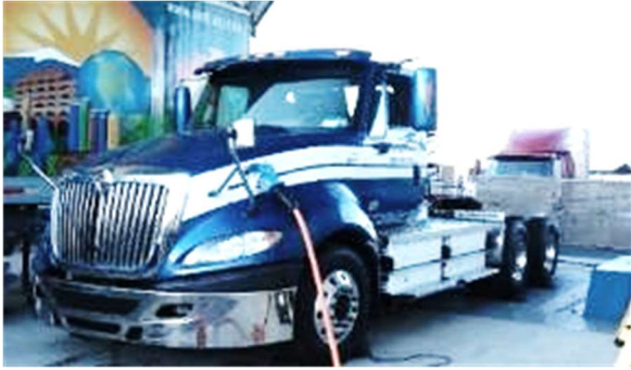
Figure 15: eTruck-1 with 180 kWh LFP 11-Pack
