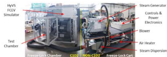
Figure 1. Nozzle Freeze-lock Chamber and Atmosphere Generating Cart at NREL
