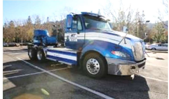
Figure 16: eTruck-2 with 280 kWh NMC 6-Pack
