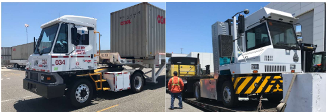
Figure 24: Kalmar and TransPower/Meritor Battery Electric Yard Tractor (Left) and CNHTC/Sinotruck and Loop Energy Fuel Cell Tractor (Right) Demonstrated at LBCT
