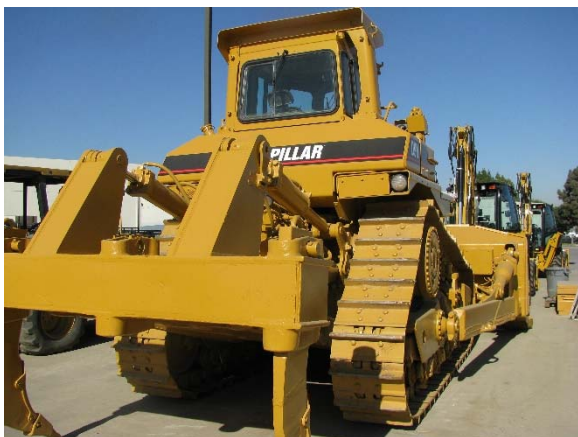
Figure 2: Caterpillar D9N Dozer Repowered to Tier 3
