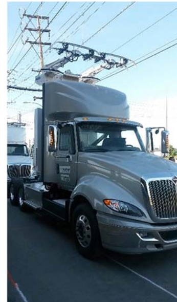
Figure 6: Drayage Truck Connected to Demonstration Catenary System in Carson
