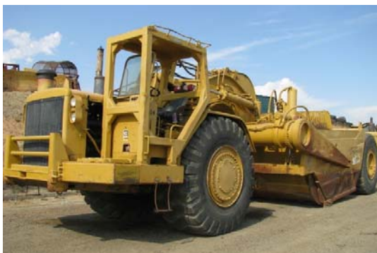
Figure 2: Caterpillar 651B Scraper Repowered to Tier 3
