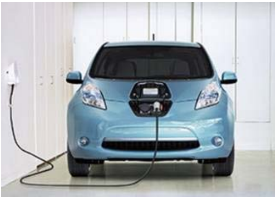
Figure 10: Residential Level 2 EV Charger
