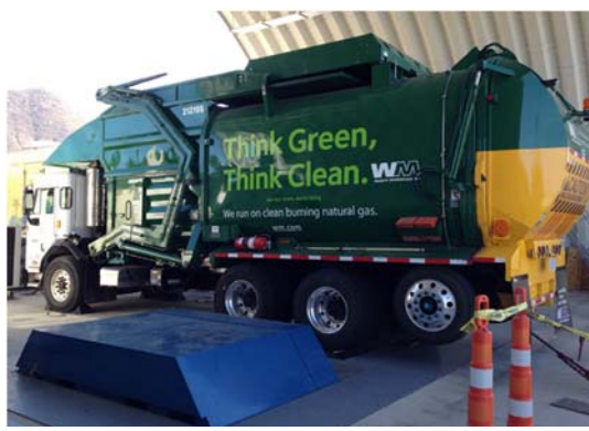
Figure 8: Truck with ISL-G-NZ Ultra Low-NOx Engine
