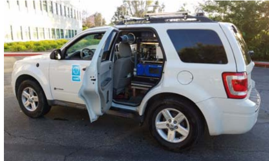
Figure 3: Quantum PHEV operated as mobile platform for South Coast AQMD Air Quality Spec. program
