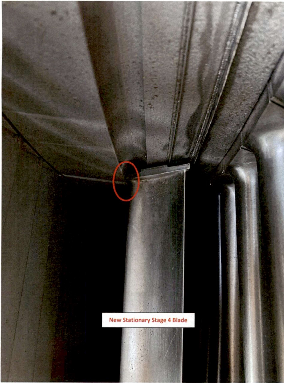
August 5 th , 2023 - Axial Clearance Interference – Required GE Repair
