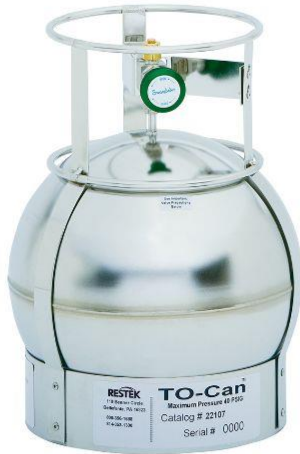
Figure D-2. Diagram of 1.4-liter SUMMA® canister
