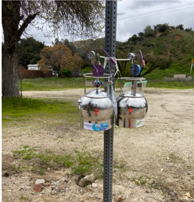
3 4 Figure 4: 24-Hour Summa Canister (and field duplicate) for Continuous 24-hour Fixed Analytical 5 Air Sampling
