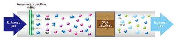
SCR catalyst decomposes NOx into the harmless  $N_2$  and  $H_2O$   $4NO+4NH_3+O_2\rightarrow 2N_2+6H_2O$
