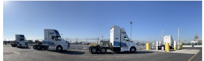
Figure 2. Port of Long Beach Station Filling Fuel Cell Electric Trucks
