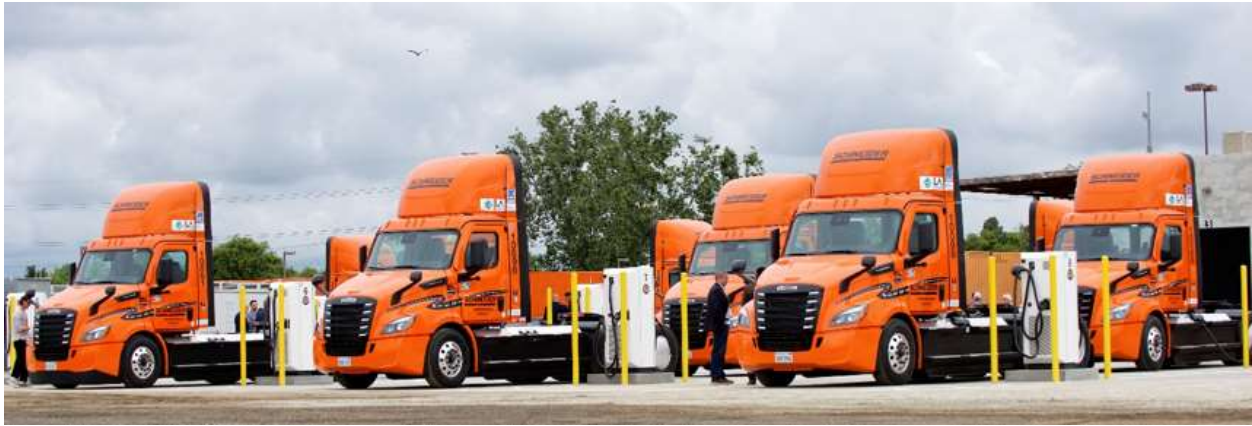
Figure 7: Schneider Deployed 50 Daimler (Freightliner) Class 8 BETs at its South El Monte Site
