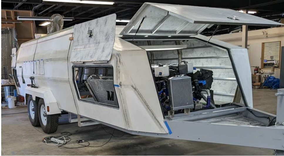
Figure 10: Custom Trailer Built to Carry First RockeTruck Mobile Fuel Cell Generator
